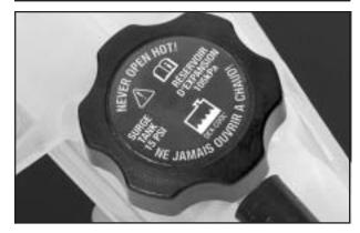
You can remove the coolant surge tank pressure cap when the cooling system, including the coolant surge tank pressure cap and upper radiator hose, is no longer hot. Turn the pressure cap slowly counterclockwise (left) about one full turn.
